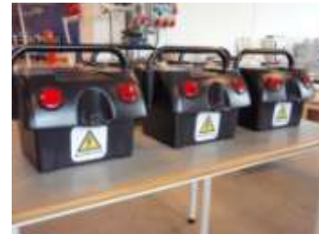
Examples of LiFePO 4 batteries for electric wheelchairs
