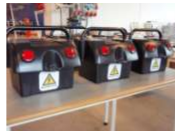
Examples of LiFePO 4 batteries for electric wheelchairs
